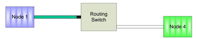
The routing switch receives the packet and checks availability of the requested output port
