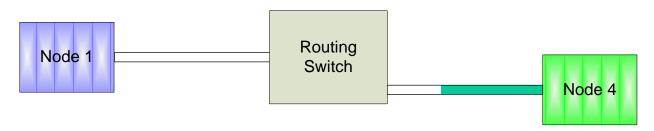
Only after the EOP has passed the occupied link is accessible for other packets again
