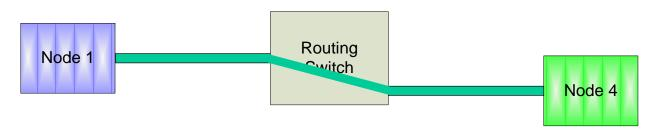
While the packet is transferred the complete end-to-end path is occupied
