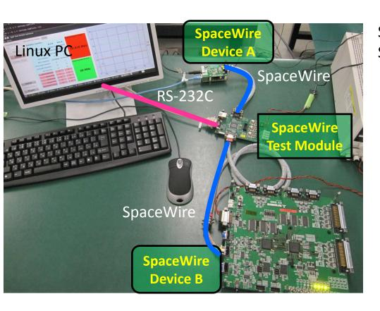
Performance test for Signaling Rate function and Statistics Counters function about Timecode were successful. SpaceWire Device A: 10.416MHz
